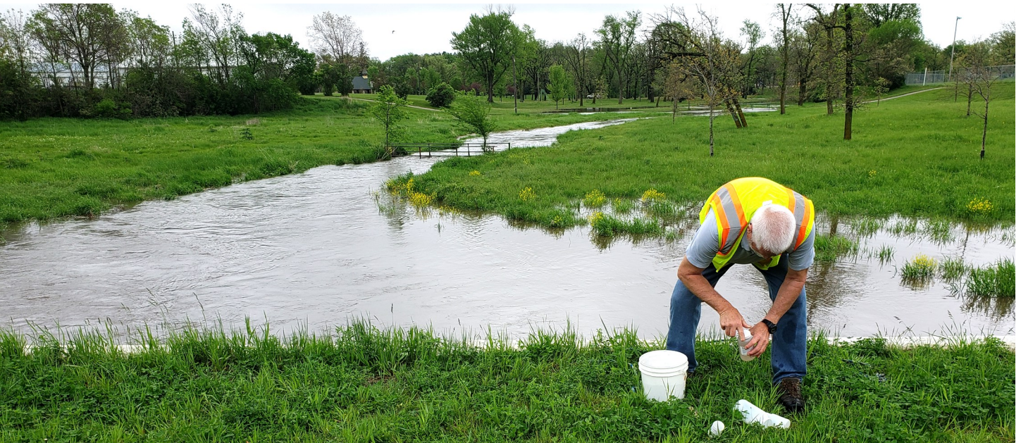
CRWD's Larry Callahan collects water samples in May 2020 from Wolf Creek after a rain storm. The site was added in 2020 to CRWD's water-monitoring program.
